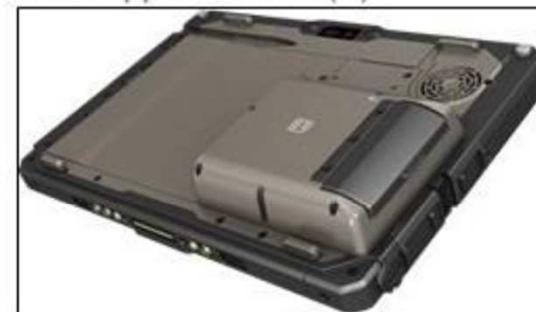
2. Bridge Battery + Smart Card Reader => Add approx. 22mm (H)
